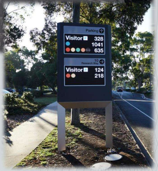
Smart Parking : Intelligent Parking Board showing number of available slots for each floor
